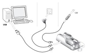
Figure 76: Charging the headset with the Travel Charger
